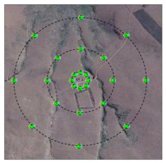
Figure 3: Calibration sampling points along three radial rings extending outwards from the cosmic ray probe (at 25 m, 100 m and 200 m). At each sample point, soil samples were taken at different depths.
